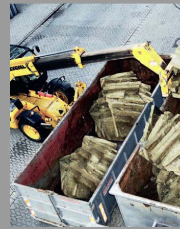
recycled stone wool briquettes
