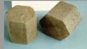
recycled stone wool briquettes
