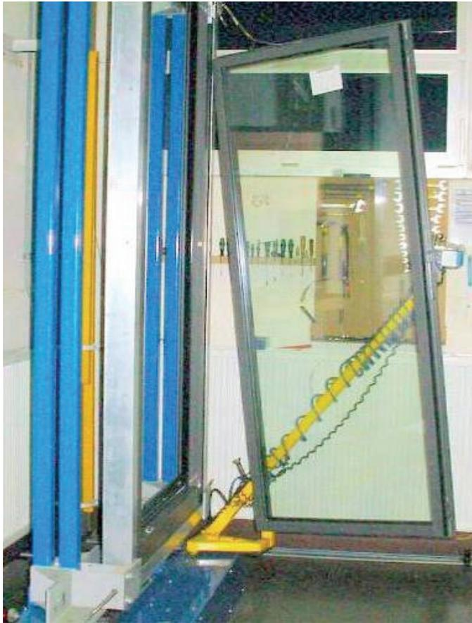
Breakage of the corner pivot during the testing procedure of 10.000 tilt and turn cycles
